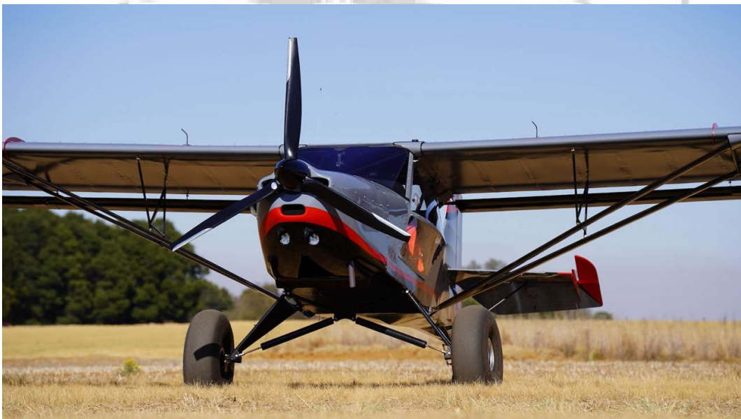
Explorer with Rotax 914 and KFA buffalo suspension
